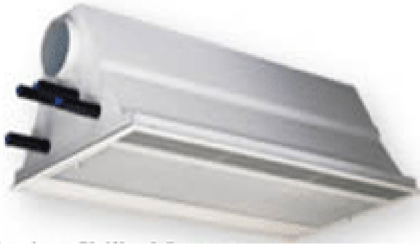
Active Chilled Beams (OA is supplied through beam to improve capacity through induction)
